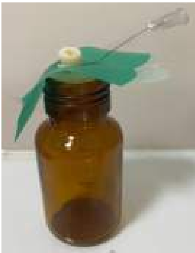
Figure 2: Final experimental setup using the Eppendorf tube system for the collection of apically extruded debris.
